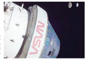
As it hurtles into Earth's atmosphere at a speed of 25,000 miles (40,000 kilometers) per hour, the gumdrop-shaped traveler will have to withstand a temperature of 2,800 degrees Centigrade (5,000 Fahrenheit) -- about half that of the surface of the sun.
